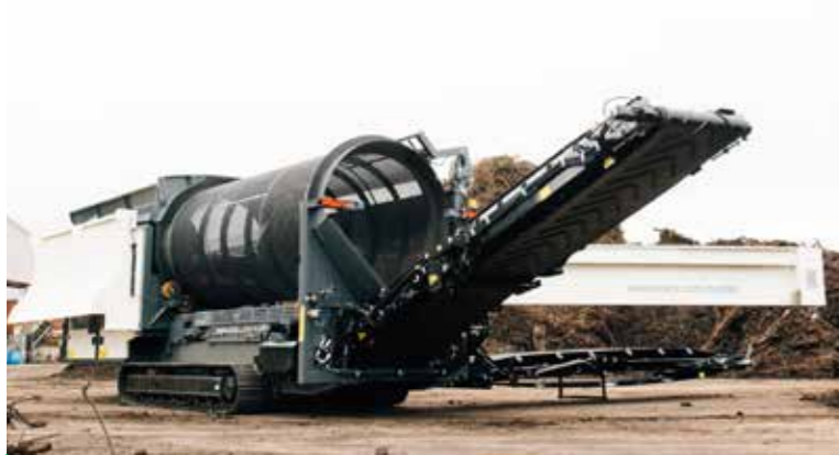
Double-sided unrestricted drum access via two large swing-out doors, enabling easy maintenance and cleaning
