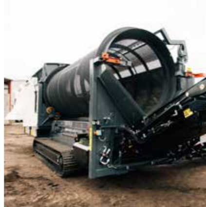
Easily replaceable 4.7m (15'5") x 1.8m (5'1") punch plate drum which is compatible with the Doppstadt SM 518
