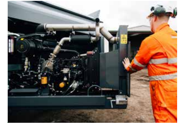
Swing out engine cradle providing operators with unrivalled maintenance access
